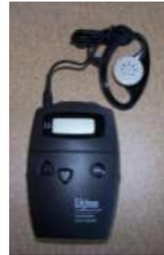
Plug ear piece into jack on left. Use dial on top to adjust volume and turn off the device
