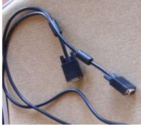
VGA cable to attach laptop to stage or floor panels
